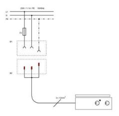
Varioshake Shaking Apparatus in 230 V with mains supply 230 V / N / PE / 50 / 60 Hz, connected through 3-pole shock-proof plug system.
