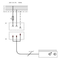
Varioshake Shaking Apparatus in 230 V with mains supply 230 V / 3 ~ / PE / 50 / 60 Hz connected through 3-pole shock-proof plug system.
