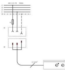
Varioshake Shaking Apparatus in 230 V with mains supply 400 V / 3  $\sim$  / N / PE / 50 / 60 Hz connected through 3-pole shock-proof plug system.
