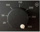
Turn the left-hand control knob clockwise to increase the shaking frequency and anti-clockwise to decrease the shaking frequency.
